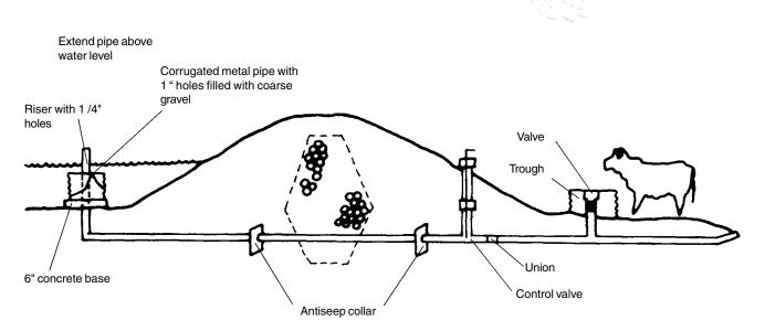
Water is piped through the dam's drainpipe to a stock water trough
